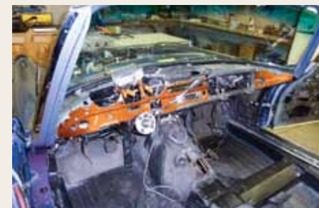
10 The interior's original rosewood trim was in fine condition and was refinished by Madera Concepts before it was reinstalled.
