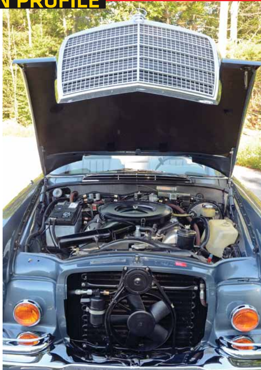
Because this 3.5 was stripped to a bare shell, there isn't one component that wasn't fully restored or replaced with a new OEM piece. The M116 V-8 was rebuilt in California and reassembled in Maine. There's an estimated $1,000 in firewall grommets alone.
