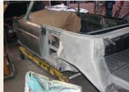
2 The unit-body car's integral rear fender had sideswipe damage and a bit of rust; it was completely replaced with new sheetmetal.
