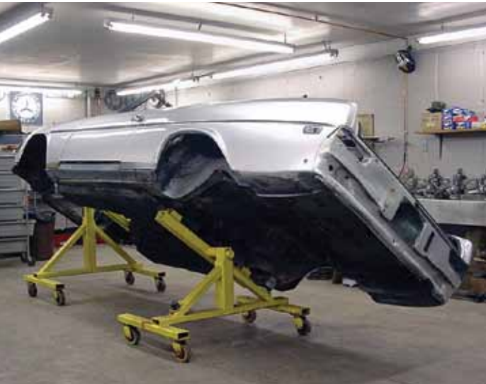
1 Gernold built a jig that raised the car to a comfortable working height, tilted for ease of access and rolled so he could readily transport the shell.
