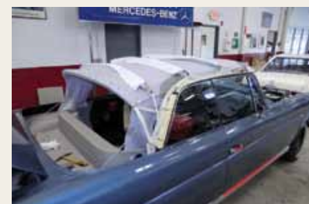
12 The convertible top bows were stripped and repainted, and the wooden supports remade, before the new multi-layer top was installed.
