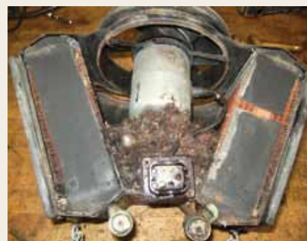
7 The bulky under-dash heater/de-froster/air conditioning blower unit was found to contain a mouse's nest.
