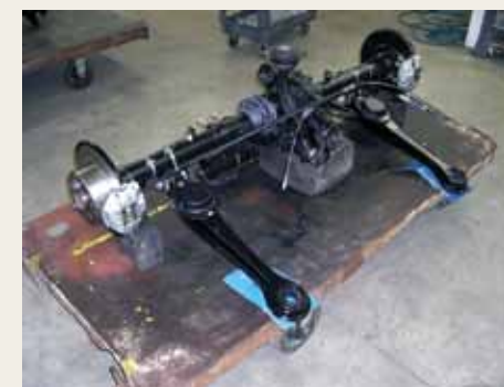
6 The rear axle assembly was completely restored with a replacement slip joint and all-new disc brake components.
